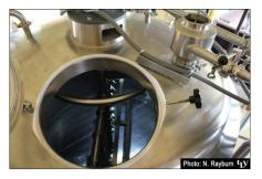
The tour began with Harvey showing us through the brewing process, explaining the function of each machine and specifics on the methods they use for Yalobusha Brewing Company's suds selections. We were shown the mash tub first because that's where brewing begins – it mixes grain evenly with 172° water and then the mixture goes
