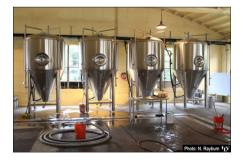
dioxide bubbles out as the yeast eats simple sugars to produce this gas along with alcohol. "It's messy," says Harvey, "but we're happy when we see the mess because it means it's doing its thing." Towards the end of the fermentation process, when the bubbling calms down, they "Cap it off, close it, and then it starts creating its own pressure. Because the more natural  $\mathrm{CO}_2$  in the beer, the better and softer the carbonation is. And we'll
